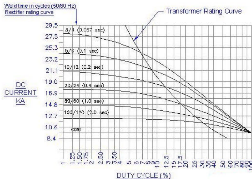
Figure 6: Typical RoMan MFDC Transformer rating curves
